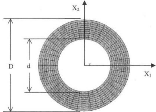
Fig. 3 Finite element model of concentric cylindrical shell
