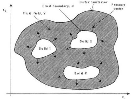
Fig. 2 Two-dimensional fluid field with cross sections of immersed  $N$  solid bodies
