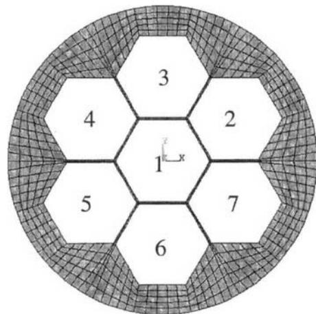
Fig. 8 Finite element model of 7-hexagons system
