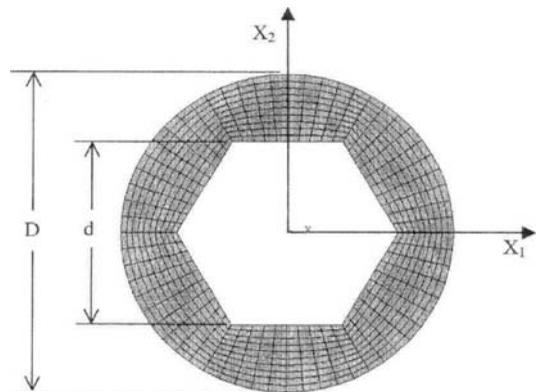
**Fig. 5** Finite element model of single hexagon system
