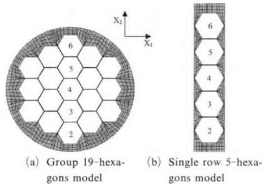
**Fig. 11** Finite element models used in analyses
